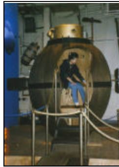
Lan demonstrates a replica of a one-man submarine powered by a hand-cranked propeller. In 1776, in the first known submarine attack, the Turtle tried but failed to sink a British warship blockading New York Harbor during the Revolutionary War.
